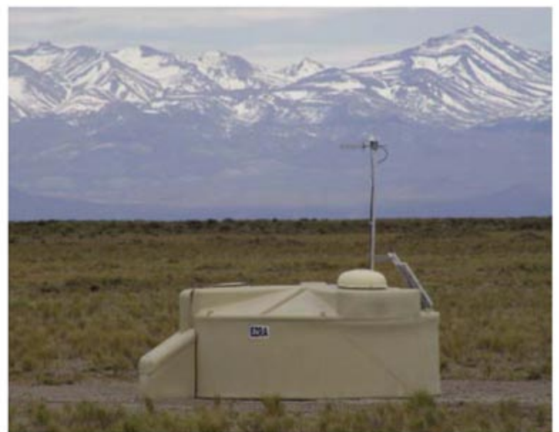
Fig. 2. A water Cherenkov tank of the Auger Observatory in the Argentinean Pampa Amarilla.
